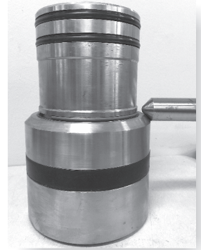
Lock-down pin in the fully engaged position.
