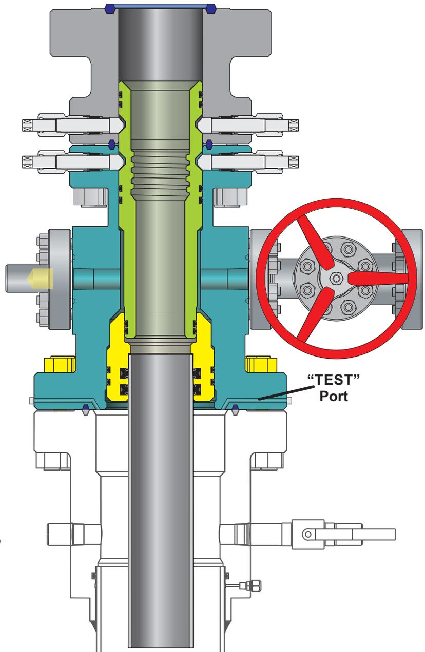
**D. Testing The Lower Master Frac Valve Connection To The Tubing Head**
