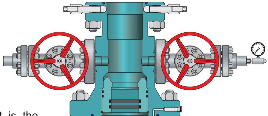
Proper cut-off height is the measured distance from the bottom flange (of the next wellhead to be installed) to the stop shoulder in the secondary seal prep.
